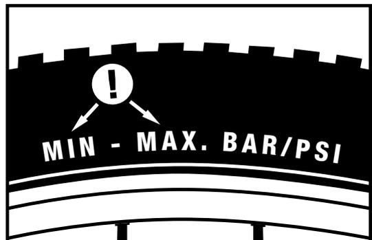
6. Verify the proper operating tire pressure as indicated on the sidewall.
